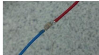
**Picture 1. Picture of Ambient Light Sensor**
