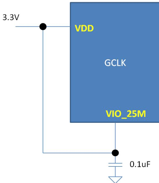
The circuit diagram shows how to resolve the boot problem by isolating VDD with a resistor and an additional 0.1uF cap
