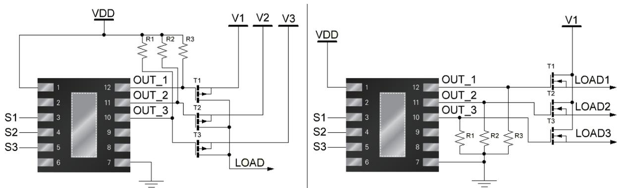
**Figure 4. Power lines control with GreenPAK2 as a driver:**
