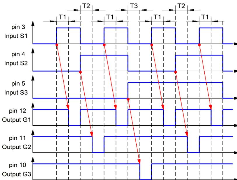
Figure 3. Timing diagram of operation of the circuit shown in Figure 4a
