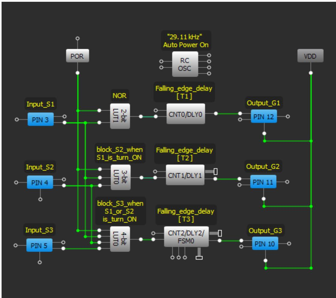
Figure 1. 3-lines GreenPAK2 driver with priority lines. The output PINs are driving P-channel MOSFET
