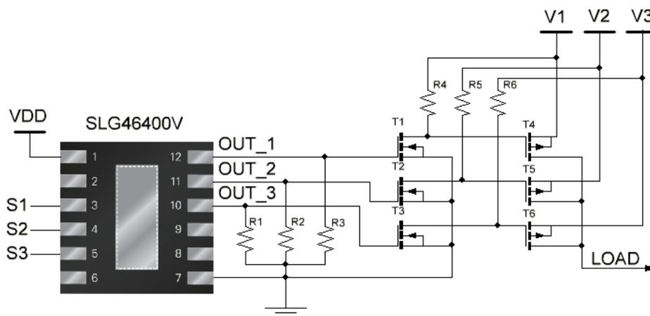
**Figure 5. Control of a high power lines using GreenPAK2 device**
