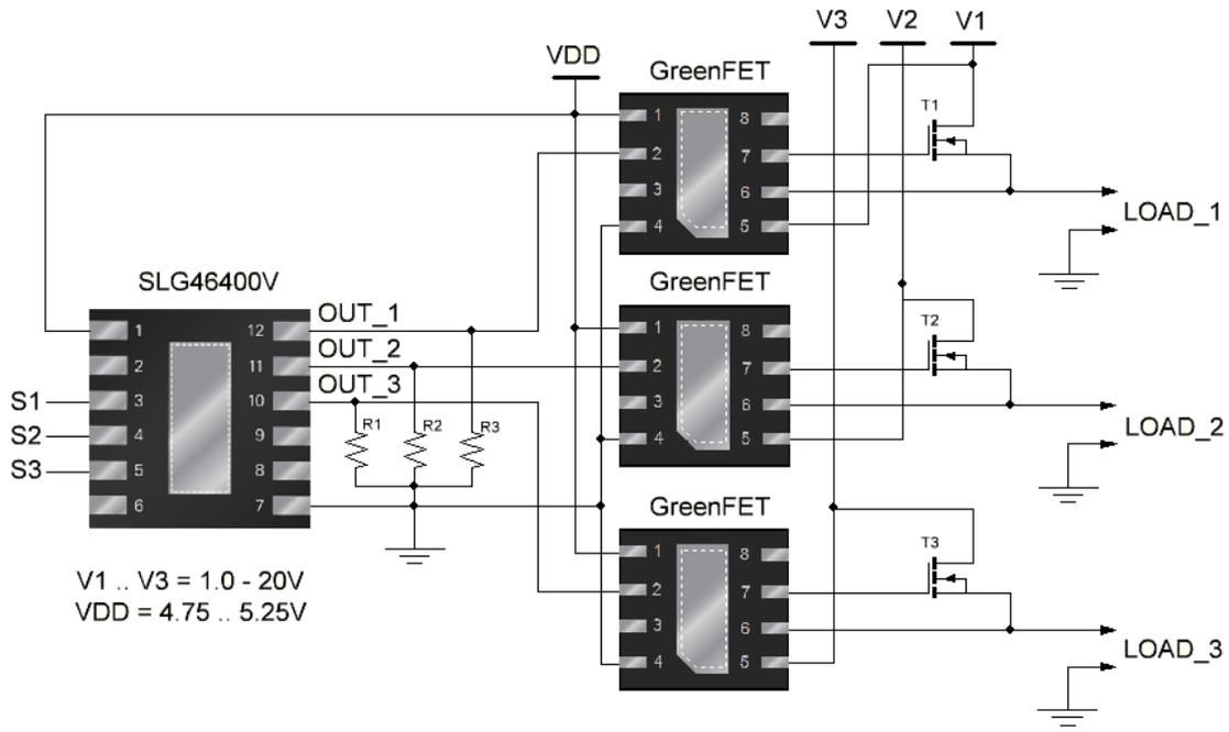
Figure 6. Control of high power lines with GreenPAK2 device and GreenFET chips as drivers
