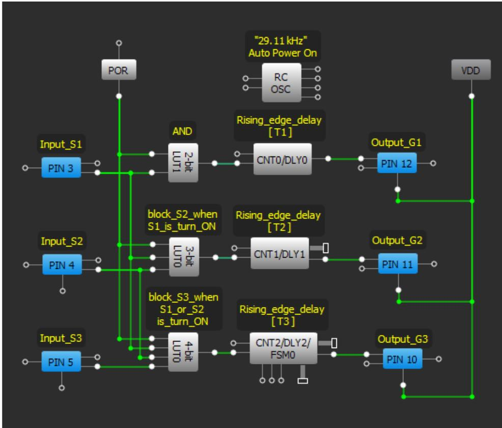
Figure 2. 3-lines GreenPAK2 driver with priority lines. The output PINs are driving N-channel MOSFET
