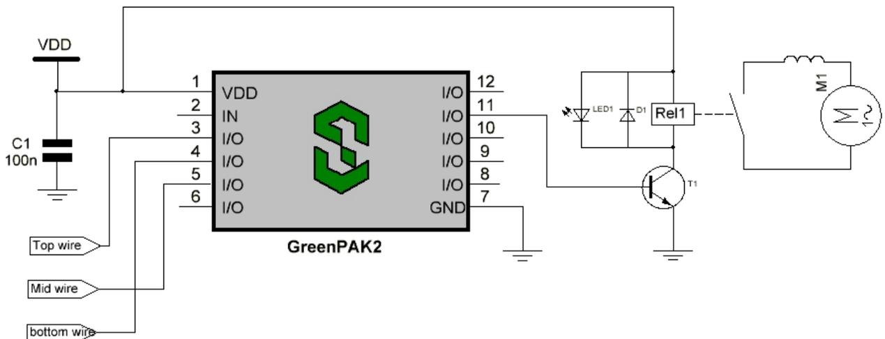
Figure 14. Applications circuit
