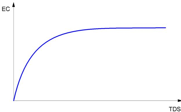
**Figure 1. Electrical characteristic of waters conductivity**
