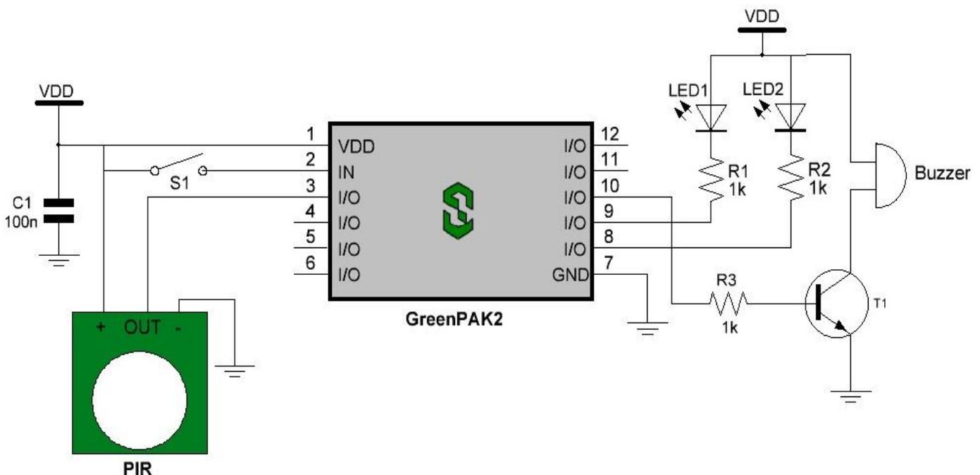
Figure 6. Typical Application Circuit
