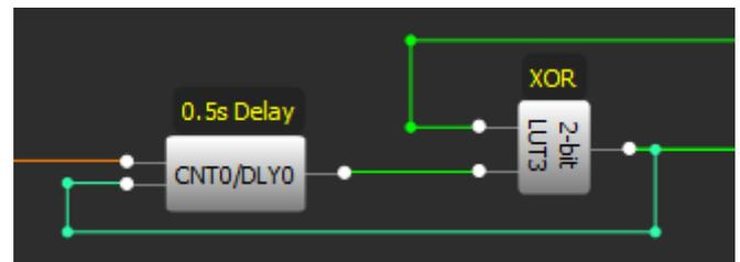
Figure 5. CNT0/DLY0 and 2-bit LUT3 in GreenPAK2 Designer
