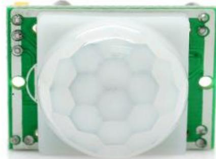
Figure 4. PIR sensor (top view)
