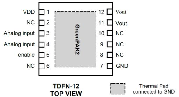
**Figure 1. Pin configuration**
