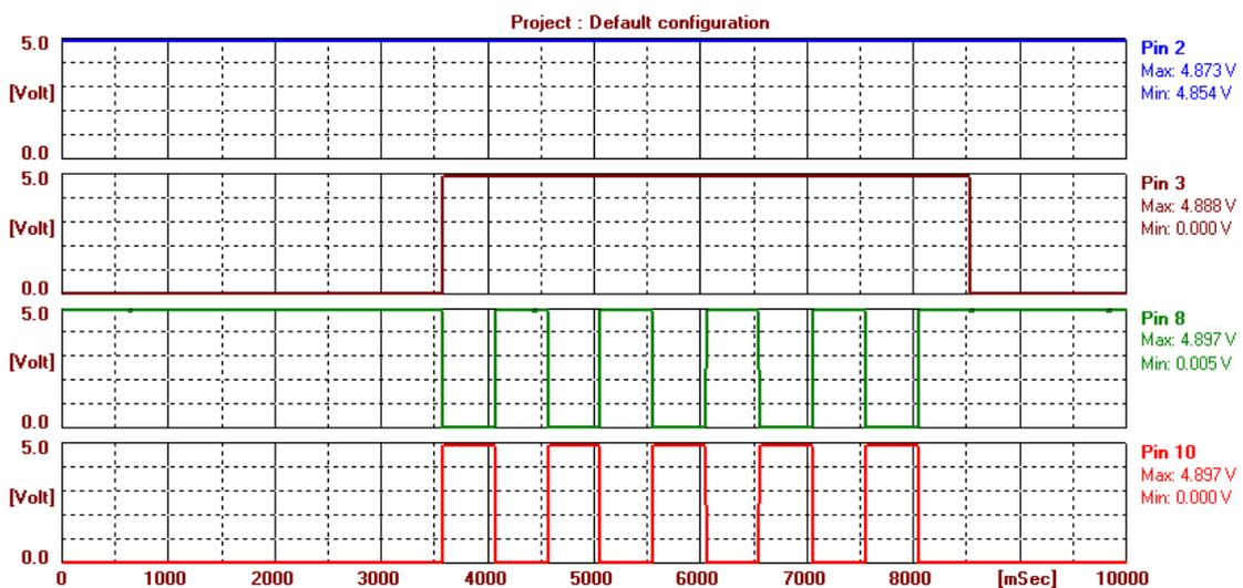
Figure 9. Functionality waveforms of subsequent motion detected
