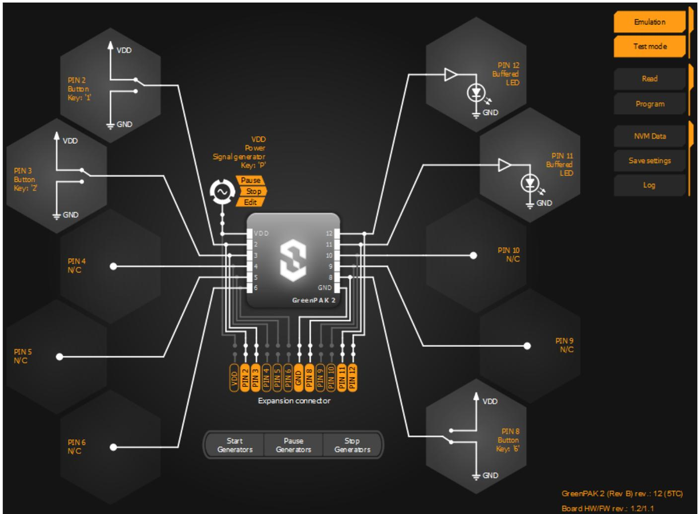
Figure 7. Configuration in GreenPAK2 Emulation Tool
