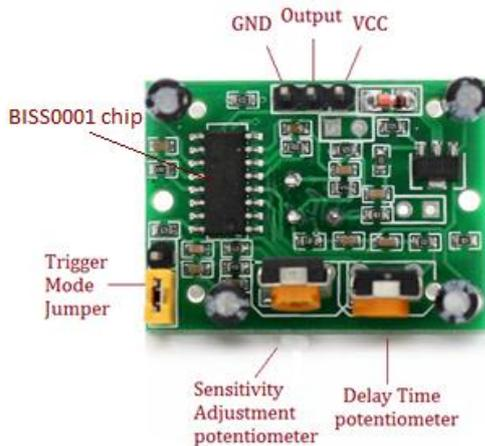
Figure 3. PIR sensor (bottom view)
