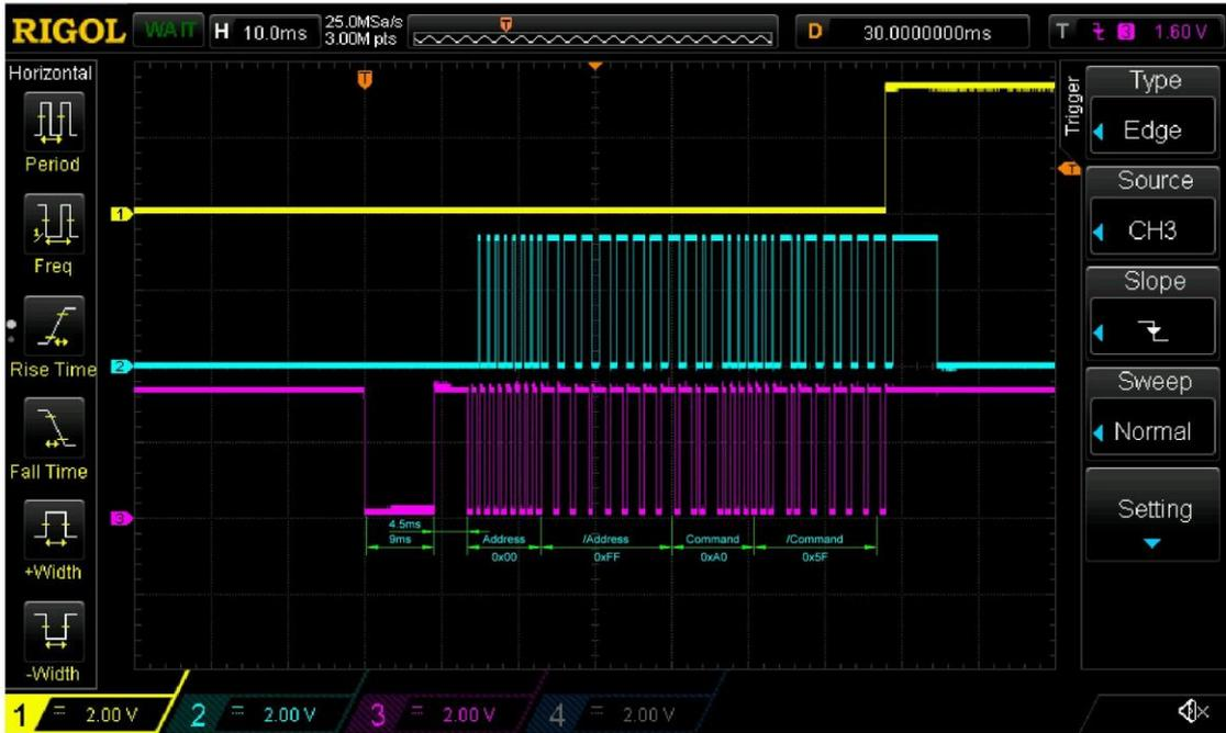
Figure 6. IR Receiver Bit Sequence
