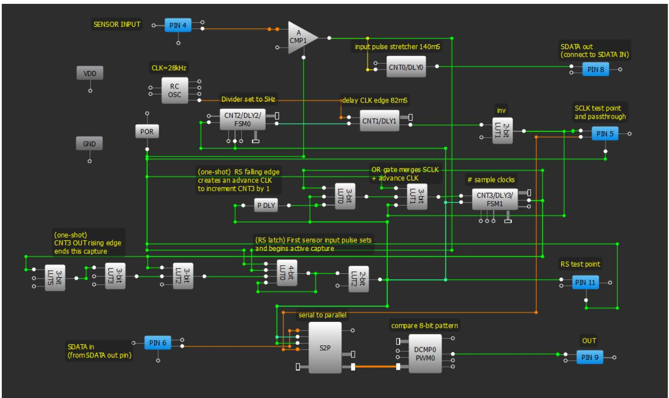
Figure 1. Complete PAK2 schematic
