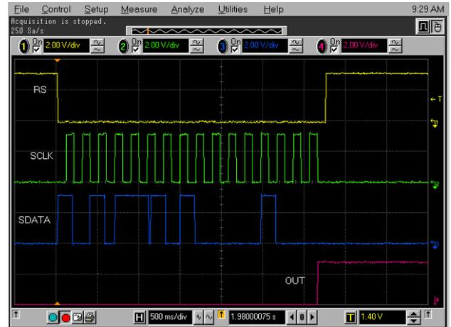
Figure 8. Waveforms of a match condition
