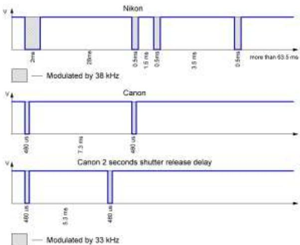
**Figure 1. Nikon and Canon wireless shutter release patterns**
