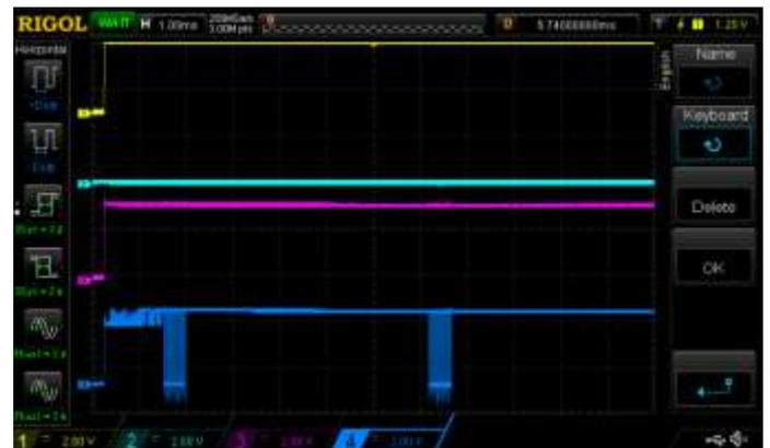
**Figure 10. Canon 2 seconds delay shutter release pattern**
