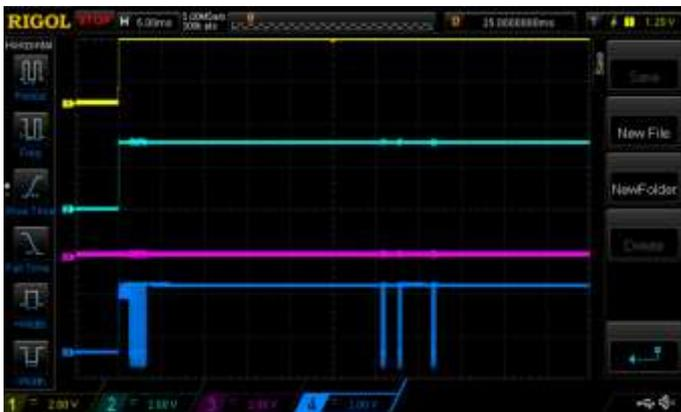
**Figure 8. Nikon (immediate only) shutter release pattern**
