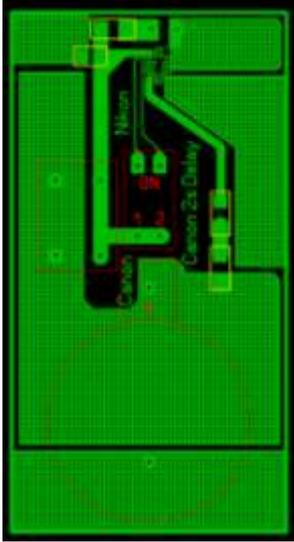
Figure 11. Wireless remote shutter release PCB layout view
