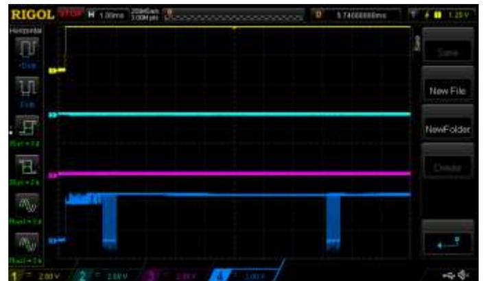
**Figure 9. Canon immediate shutter release pattern**
