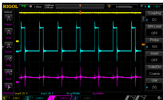
Figure 5. Device functionality then SPI code 192 at VDD 5.5V
