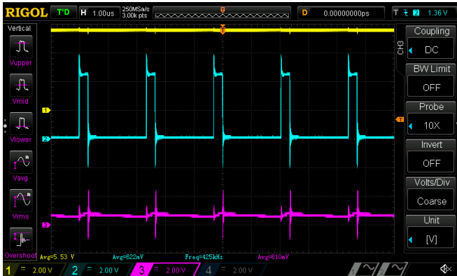
Figure 7. Device functionality then SPI code 128 at VDD 5.5V
