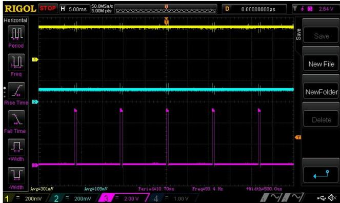
**Fig 4. Timing waveforms for servomotor position -90 degrees**
