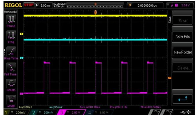
**Fig 5. Timing waveforms for servomotor position 90 degrees**
