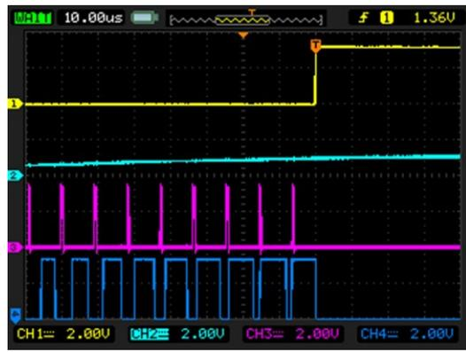
Figure 9. PWM generator turns off
