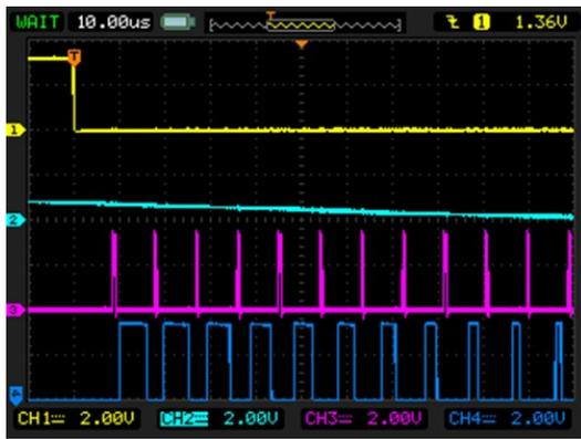
Figure 8. PWM generator turns on
