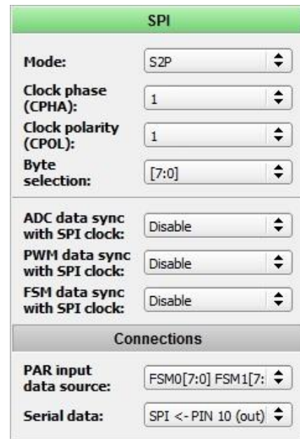
Figure 9. SPI block configuration
