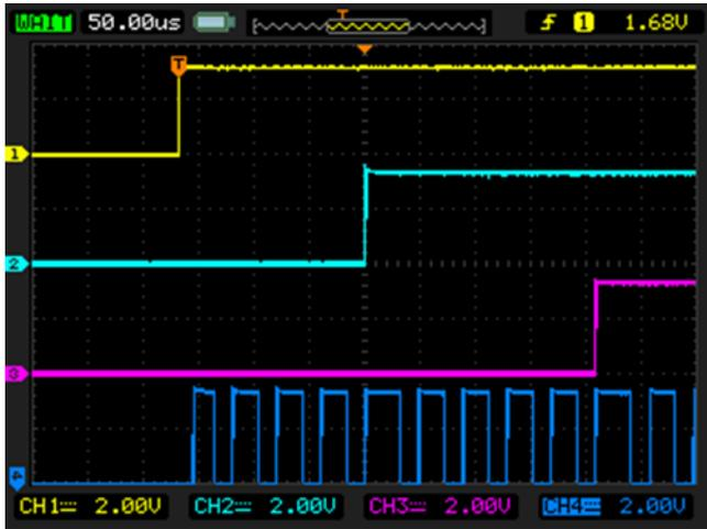
**Fig. 4. Series Connection of Delay Cells waveforms (blue=RCOSC)**
