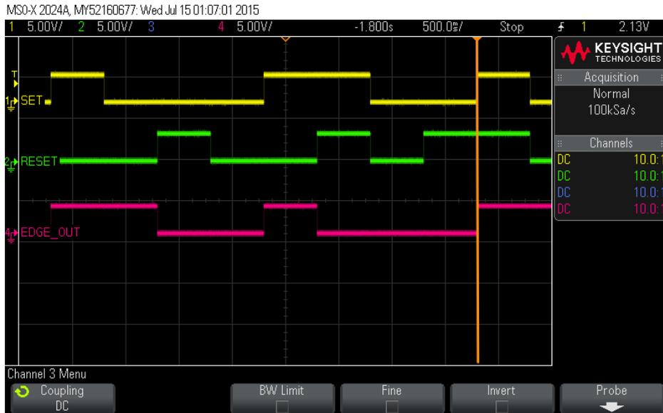
Figure 2. Level Triggered RS Latch Timing Diagram
