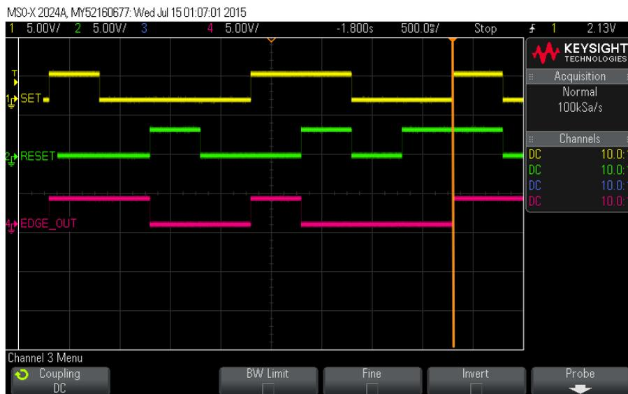
Figure 4. Edge Triggered RS Latch Timing Diagram
