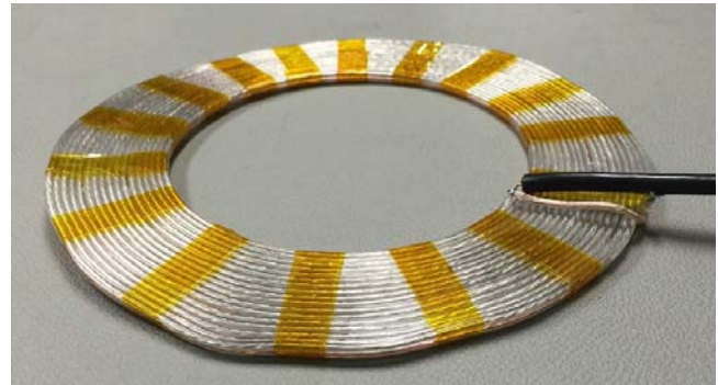
Fig 1b. Example search coil
