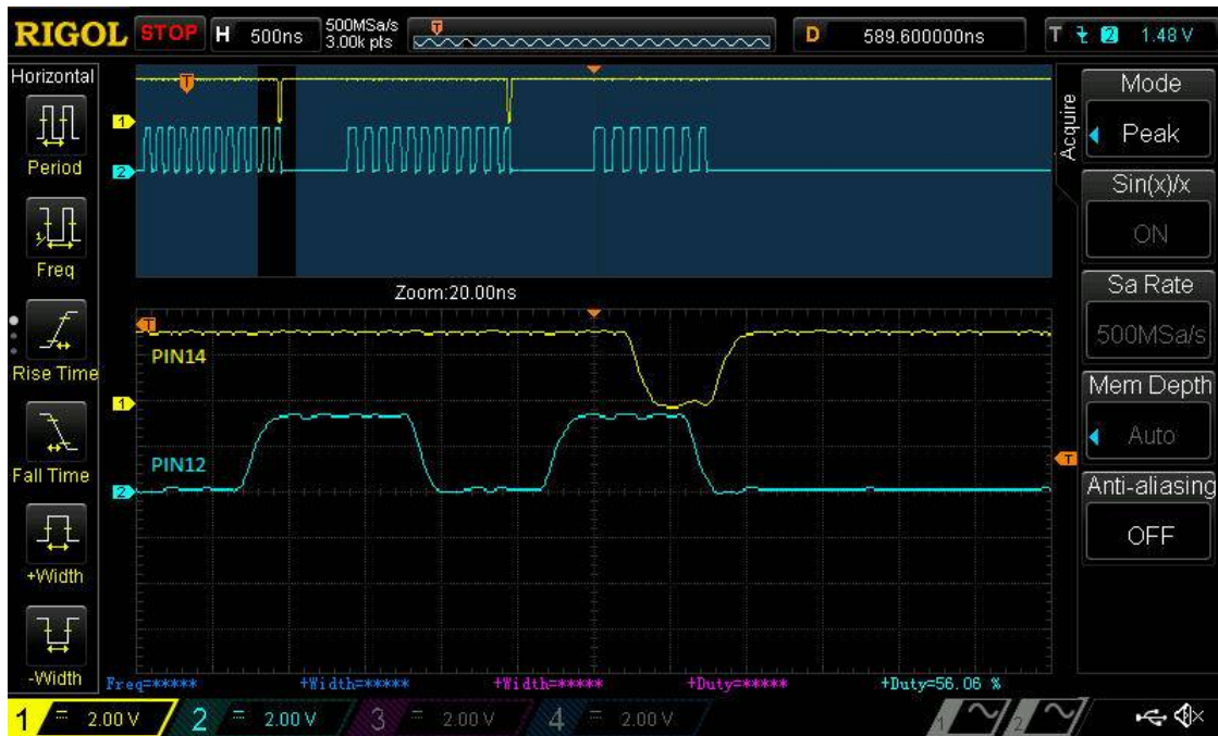
Channel 1 – 2-bit LUT0 output; Channel 2 – Ring OSC output
