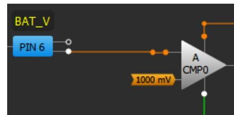
**Figure 1. Analog In PIN6 hooked up to ACMP0**
