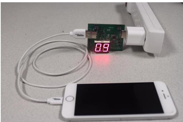
**Figure 9. Current Monitor Board Measuring Phone Charge Current**
