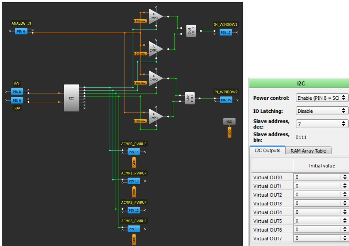
Figure 1. Dual window comparator design viewed in the GreenPAK Designer and I2C block configuration
