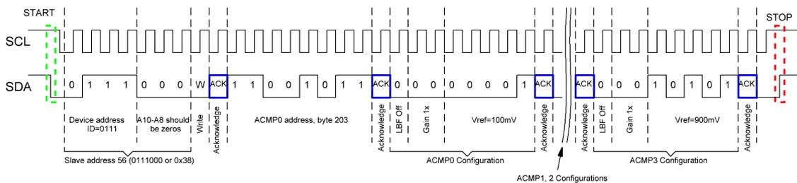
**Figure 3. ACMPs  $V_{ref}$  programming via I2C. Timing Diagram**
