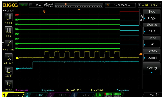
Figure 6. 1us scale of Data Byte 0xFF
