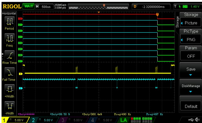
Figure 3. I2C Command [0x00, 0xF4, 0x00]
