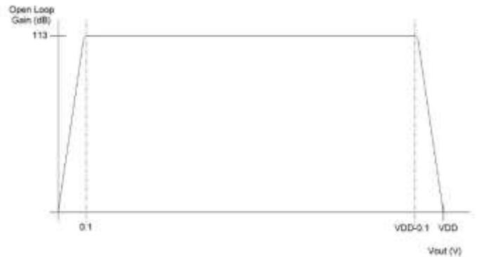
**Figure 7. AOL vs VOUT Characteristics for SLG88104V**
