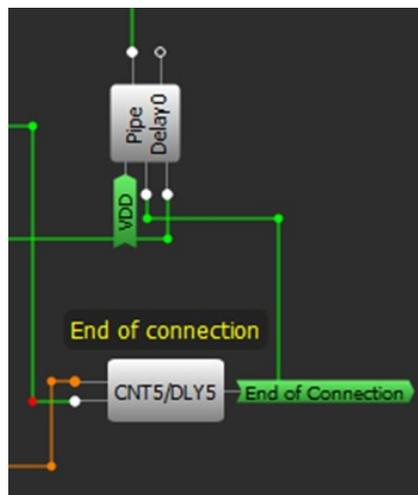
Figure 8. Applied delay to the end of the connection signal
