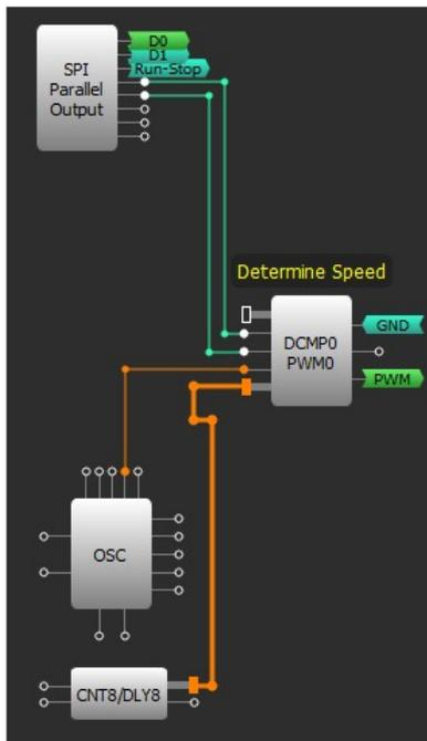
Figure 9. Connections of S1 S0 bits
