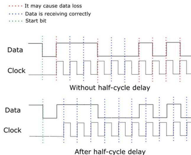
Figure 6. Timing (Before and after half-cycle delay)
