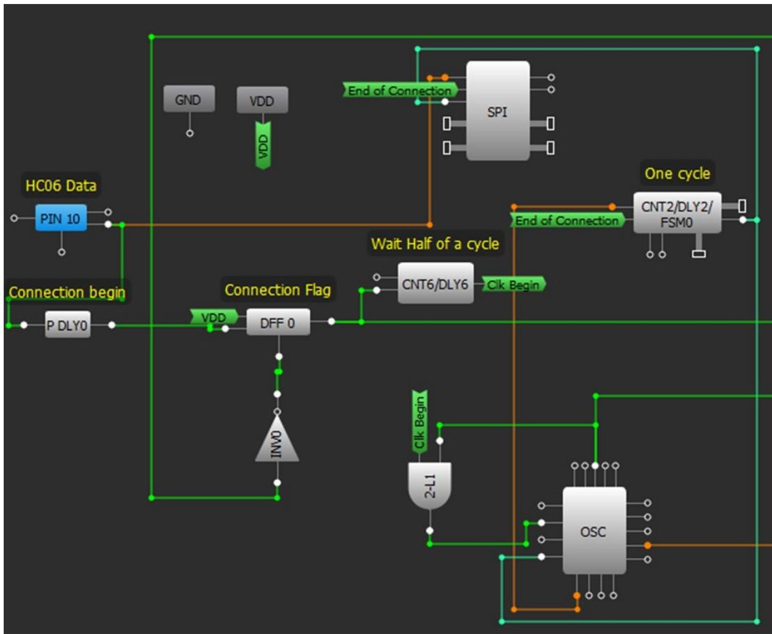
Figure 7. Connections of Counters
