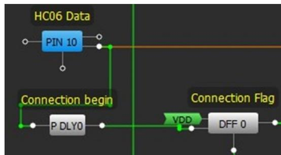
Figure 5. Start Bit Detector and Connection Flag
