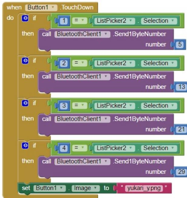
Figure 4. Programming blocks of go forward button
