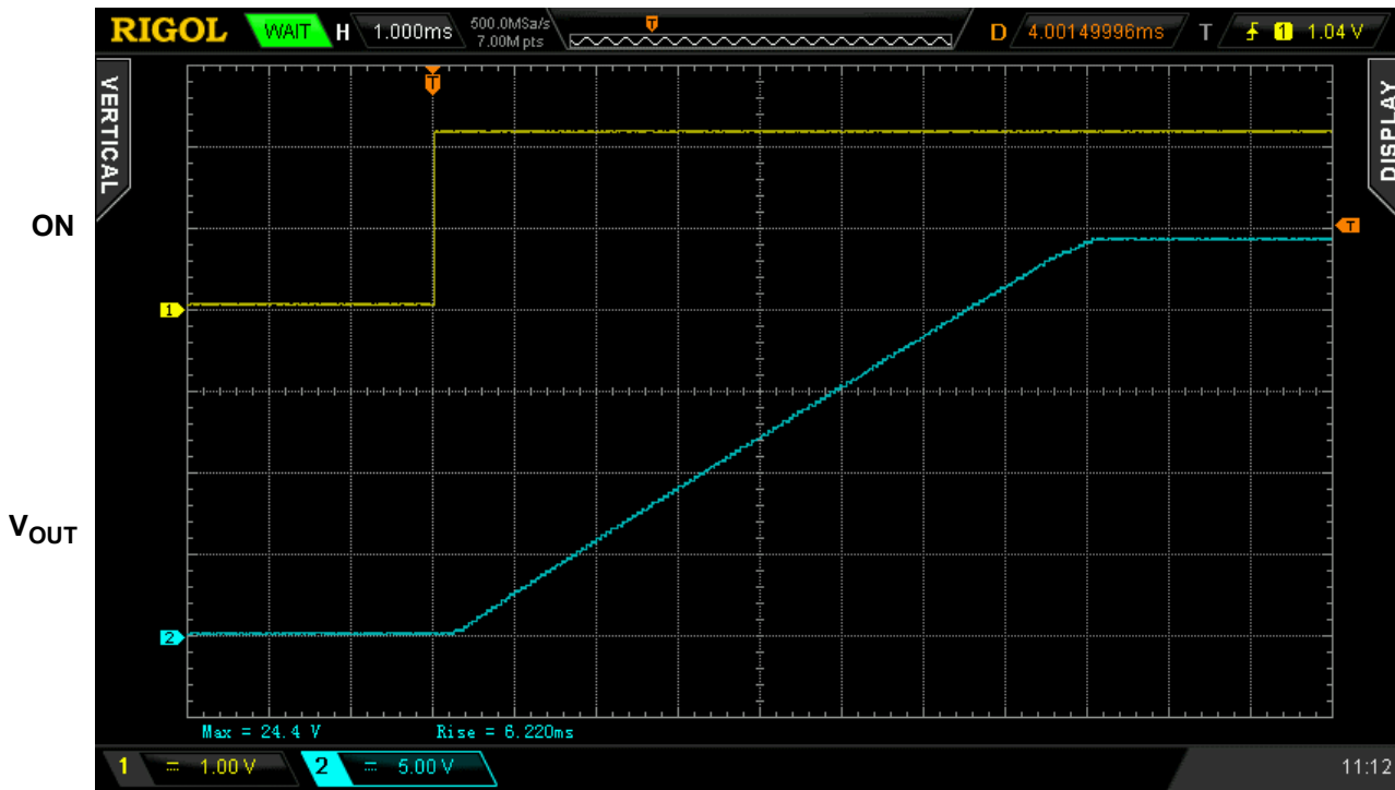
Figure 3. Typical Turn ON operation waveform for V_{IN} = 24\text{ V} , C_{SLEW} = 10\text{ nF} , C_{LOAD} = 10\text{ }\mu\text{F} , R_{LOAD} = 100\text{ }\Omega
