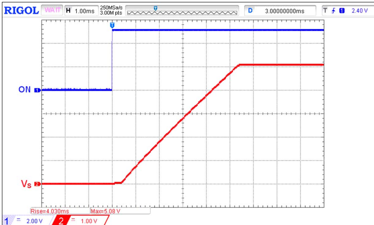
Figure 2. Typical Turn ON operation waveform for V_D = 5\text{ V} , C_{SLEW} = 12\text{ nF} , C_{LOAD} = 10\text{ }\mu\text{F} , R_{LOAD} = 20\text{ }\Omega
