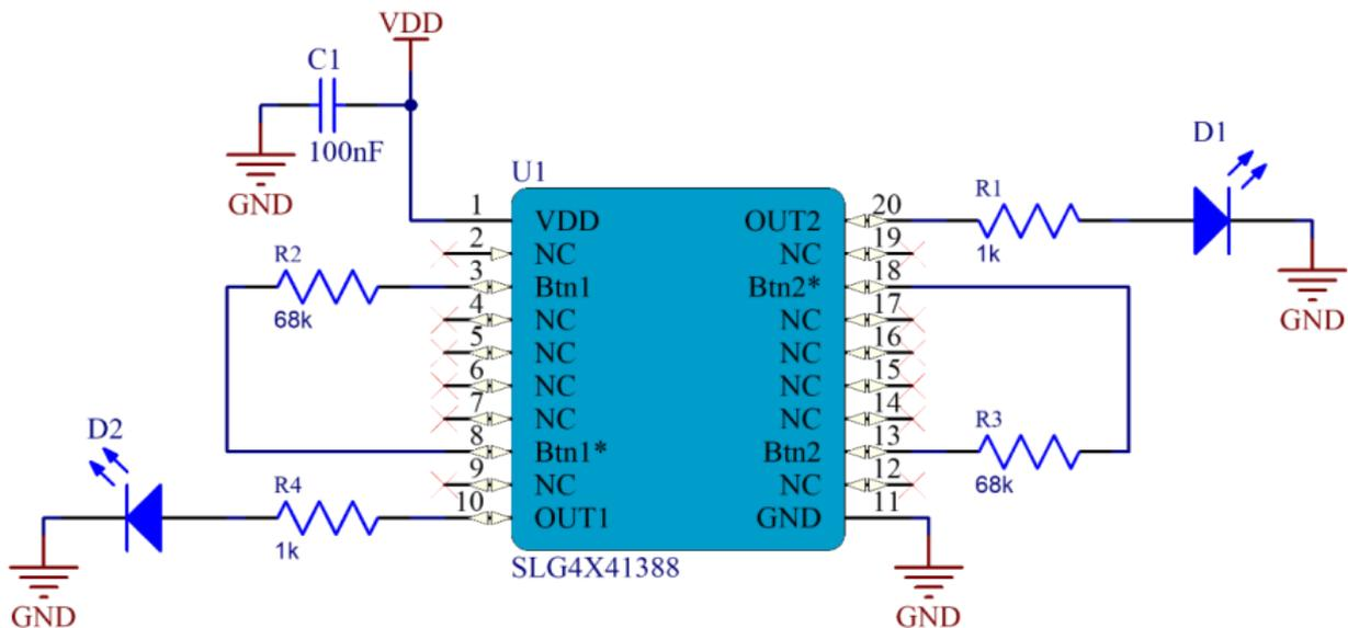
Figure 2. Touch Sensor circuit
