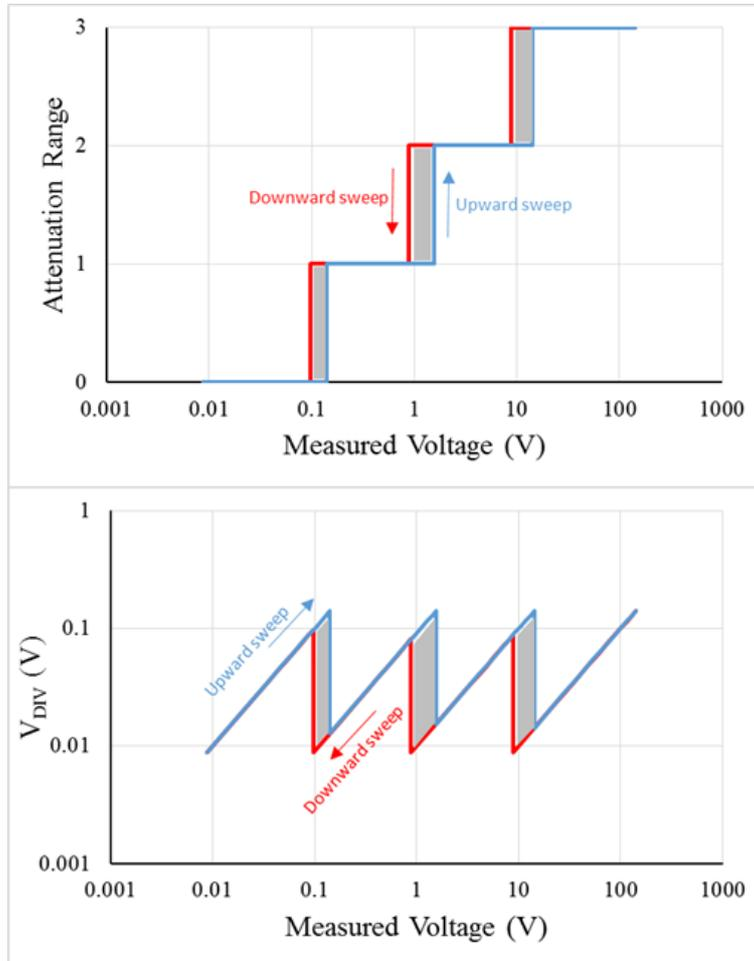
Figure 6. Attenuation range and V<sub>Div</sub> as functions of V<sub>Meas</sub>
