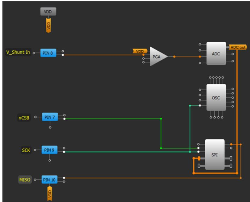
Figure 2. Part 1 of the SLG46621V's internal connection diagram
