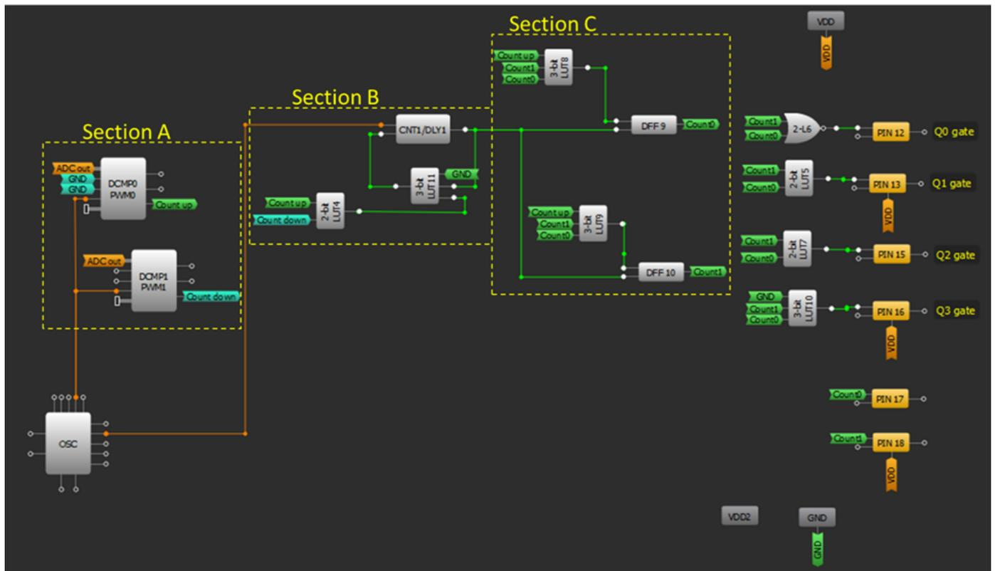
Figure 3. Part 2 of the SLG46621V's internal connection diagram
