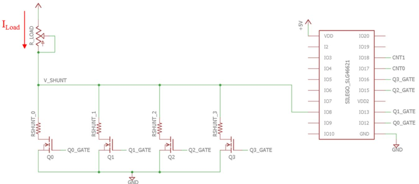
Figure 1. Autoranging ammeter test circuit
