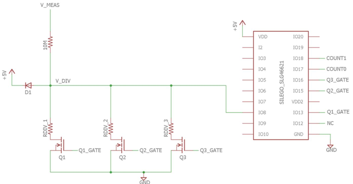
Figure 5. Autoranging voltmeter test circuit
