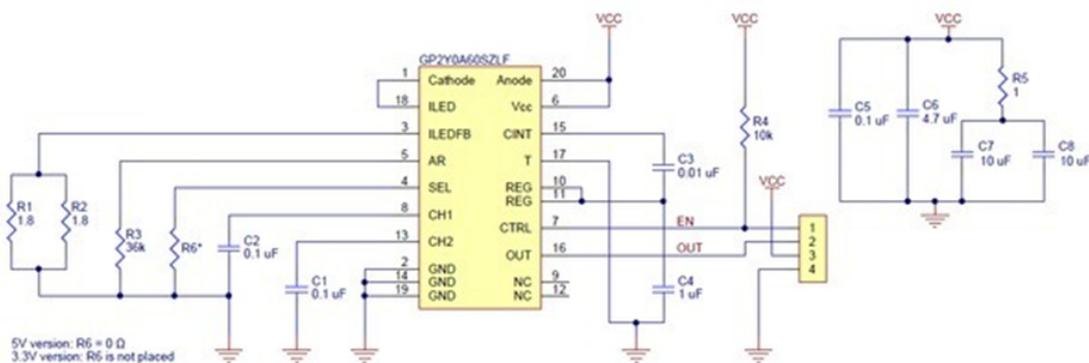
Figure 2. Sensor circuitry
