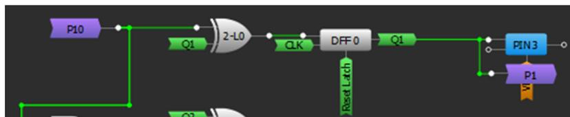
Figure 8. First Block of 4-Bit Counter
